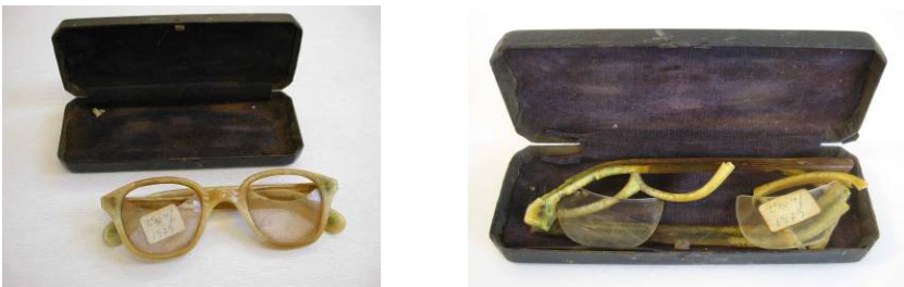
Figure 1 - Two pictures of the same cellulose nitrate spectacle frames, in 2002 in visibly good condition (left) and in 2014 in a degraded state (right). (Source: Photographs courtesy of Yvonne Sbashoua, National Museum of Denmark)
